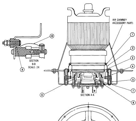
CROSS-SECTION OF SK-300A SHOWING 4CX5000A WITH SK-306
